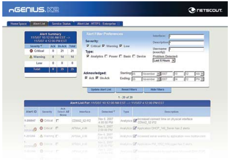
The nGenius K2 Alert List displays the time, location, severity, and the links and applications affect by anomalous behavior, as well as a description and links to supporting charts, providing the evidence necessary for fast problem resolution. It also provides rich filtering capabilities.
